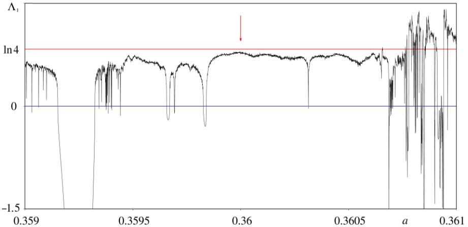
Fig. 3. Graph for the largest Lyapunov exponent of the Poincaré map versus the parameter  $a$ . An arrow indicates situation corresponding to the Smale-Williams attractor with parameters (2)
