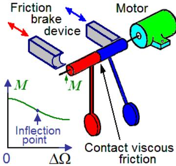
Fig. 1. A system of two Froude pendulums: the motion of one and the other pendulum is decelerated alternately by attaching a brake shoe providing suppression of the self-oscillations
